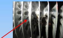
Close-up of coil after conventional cleaning (note: black tar like substance is biofilm)
